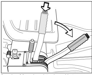
Lowering of the cutting unit (cutting position)
